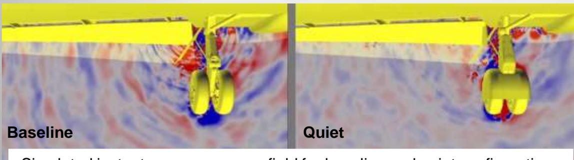
Simulated instantaneous pressure field for baseline and quiet configurations
