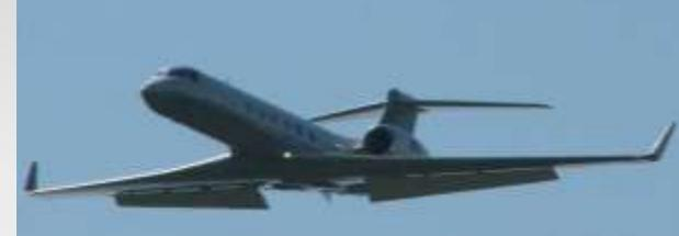
Flap 39°, main gear deployed configuration
