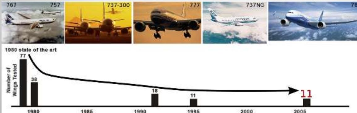
Inability to further reduce number of tests due to deficiency in modeling of turbulent flow physics
