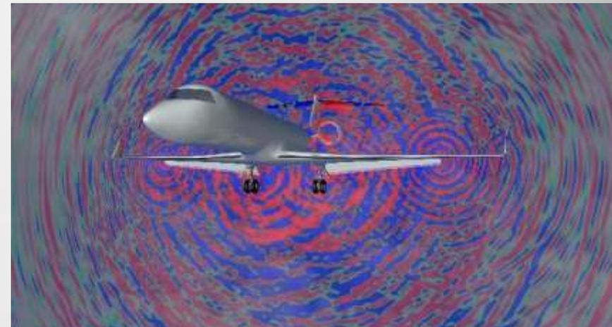
Simulated radiating pressure field for baseline configuration
